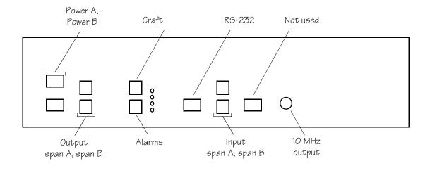
Figure 9. Optional Wire-Wrap Panel Rear Panel Connectors
